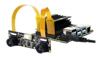
Two Sony IMX219 sensors capable of 3280x2464 resolution images.
