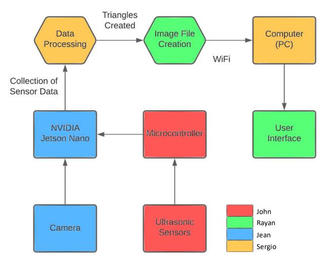
Software Block Diagram for 3D scanning Device
